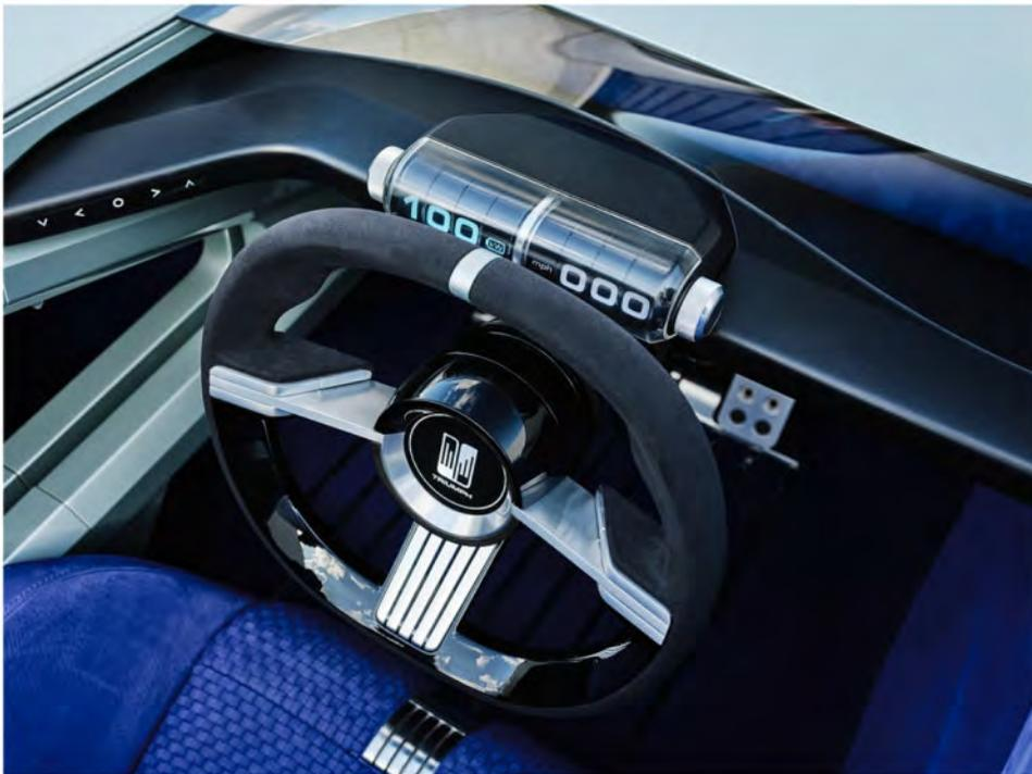
A self-centering dial in the steering wheel displays all vital information while a central binnacle will show road speed, charge levels, and battery range. The spoked steering wheel, which pays tribute to the ‘Jabbeke’ TR2’s wheel in period, will be where the driver can access driving modes, data and the car’s navigation system.
