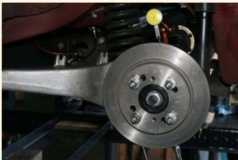
Disc runout checked with a dial gauge
