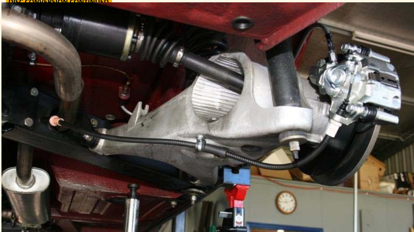
Brake installed with handbrake cable secured to trailing arm
