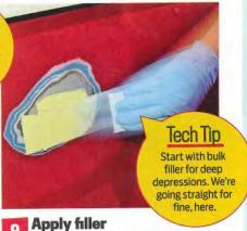
Make sure the area is dust-free. Wipe the spreader with a clean cloth. Scrape a quantity of filler from the edge of the mixing board. Apply it to the edge of the area and smoothly spread it across to avoid air bubbles. Repeat, overlapping a little.
