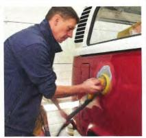
Clean the dent and surrounding area with panel wipe. Hand- or power-sand the dent and note the number of paint layers. If there are only a few, only the immediate area needs to be bare-metalled. If there are lots of layers, bare-metal the whole area.
