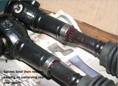
The second is that the splined sliding joints lock up under load which causes an obvious rear end twitch during cornering.
