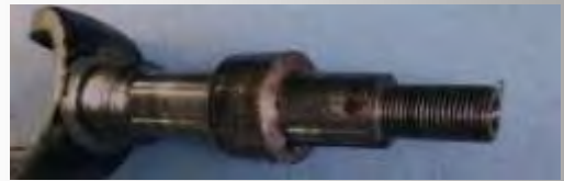
Mark 1 2000 axle removed before breakage occurred
