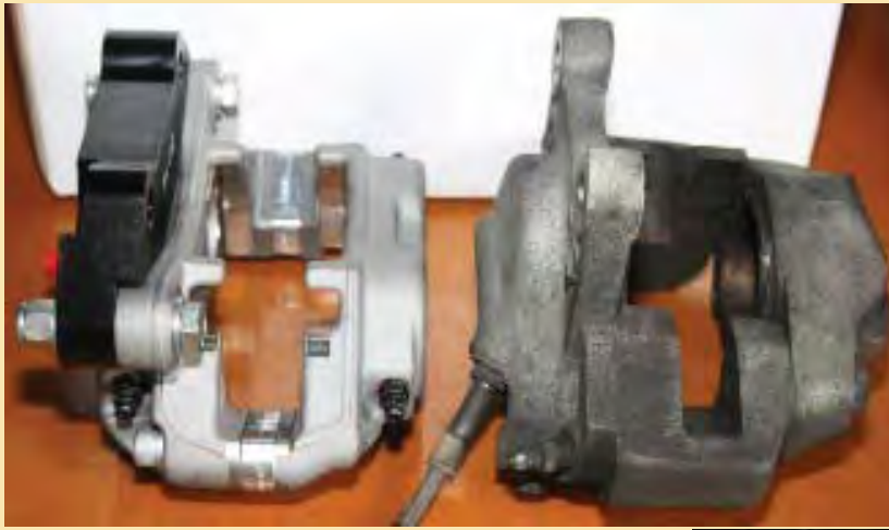
Replacement caliper is thicker than the original
