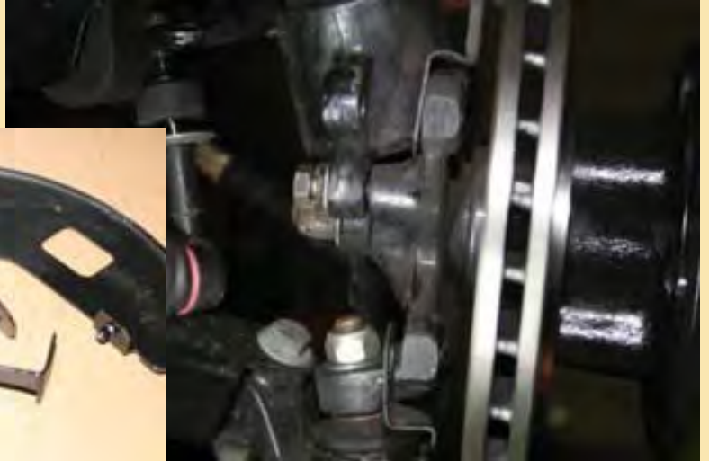
Dust shield lugs prevent correct fitting
