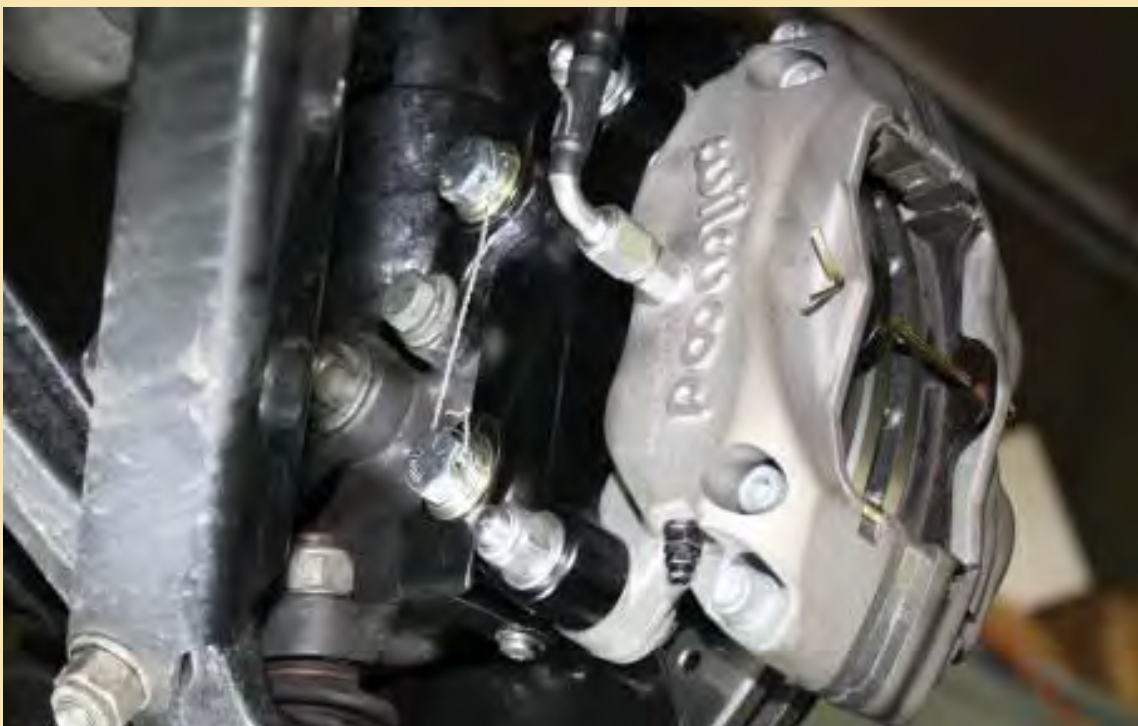
Final fitting with attachment bolts lockwired into position
