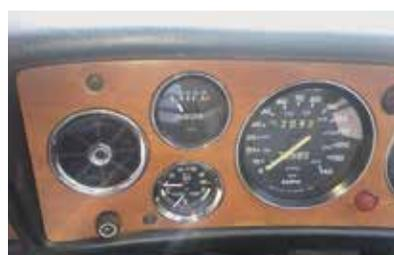
Australian Stags have a metric speedometer and odometer ....
