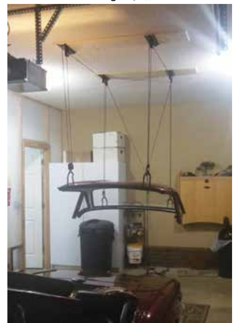
Yet another attempt (on a TR6) although the bicycle-type hooks look a little weak
