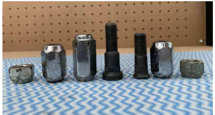
This illustrates the standard and longer stud and wheel nut options.
