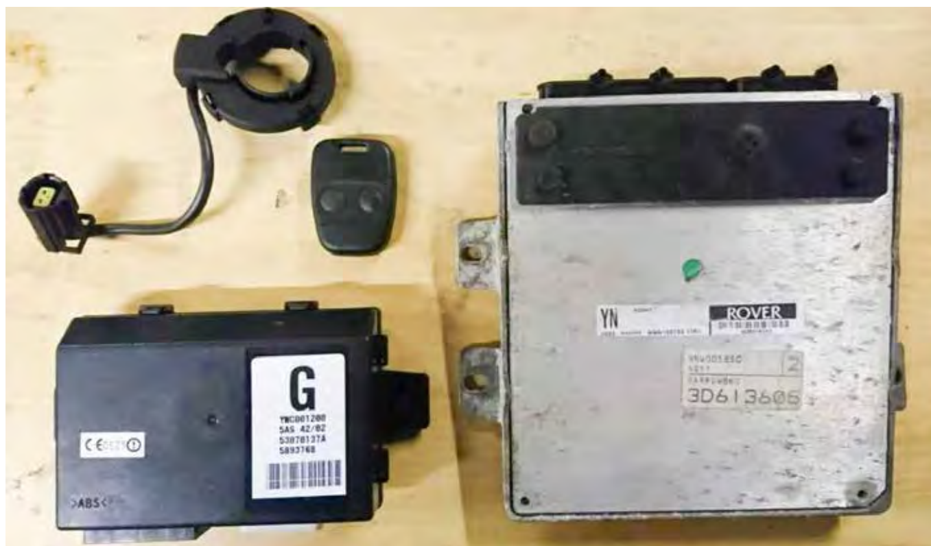
Shown is an early set of key fobs, Lucas 5as immobiliser and ECU.
